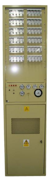
This very high performance unit stands over 2.2m high, and is home to two 3/4HP compressors. Using timers and pressure switches, the compressors are controlled to run alternately when the demand for air is within the capability of one.
