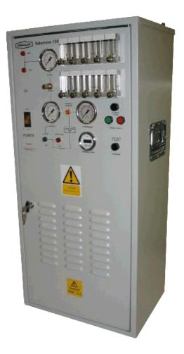
The 12437/H uses an efficient 1/3 HP compressor, to fill its integral receiver to a pressure in excess of 60 p.s.i. The receiver is a high capacity metal item, which has been tested and Lloyds certified at three times the units' maximum working pressure.
