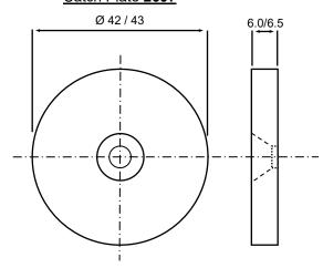
Fix with M5 countersink screw, (not supplied).
