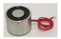
This magnet exerts a holding force of approximately **40 Kgf** perpendicular to any steel plate (see accessories) with which it is in contact, assuming nominal voltage, and coil at working temperature rise of 60°C in an ambient of 20°C.
