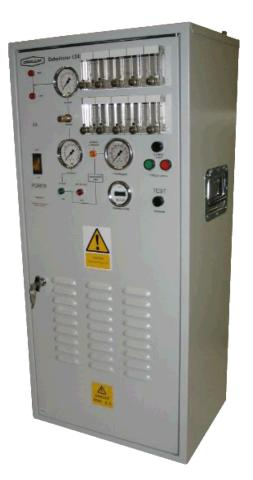
The 12437/H, designed for cable pressurisation applications, has proved successful in numerous aerial and waveguide applications, and a low pressure version has evolved. This unit is the same as its higher pressure counterpart, but for an output regulator, and gauge which are more accurate within the 0.5 to 3 p.s.i. pressure band.
