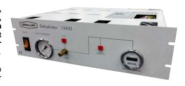
reducing running costs. Complete with an output pressure regulator and gauge, the 12435 is delivered ready for connection to up to 3 waveguide tubes, via ¼" outlets on the rear of the unit. Standard alarm monitoring facilities include our humidity detection equipment and low pressure alarm switches. Alarm conditions are communicated both visually and remotely via a hard-wired connection.
