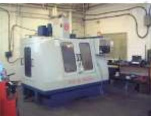
Horizontal Machining Centres with up to (X) 650mm (Y) 650mm (Z) 550mm and Auto Pallet Change Facility, Laser Tip Break Detection and Probing
