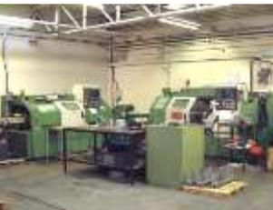
350 Dia. x 500 Long with 70mm Dia. Magazine Bar Feed Capacity, 'Y' & 'C' Axis with Live Spindle Tooling
