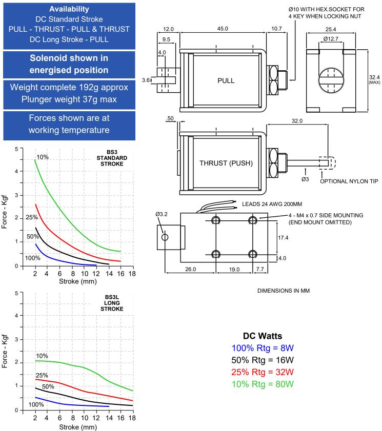
\*\* Please note: Fixing, plunger coupling, thrust rods and lead length can all be customised \*\* We reserve the right to alter or amend designs without prior notice.
