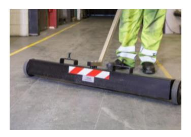
The Forklift Truck Magnetic Sweeper's heavy duty magnetic design effortlessly picks up ferromagnetic shards, nuts, bolts, pins and nails (non-magnetic materials such as aluminium, copper, some stainless steels, etc are not attracted to magnets and remain uncollected). In areas where tyre punctures are known to occur due to ferromagnetic materials piercing the tyres, the Forklift Truck Magnetic Sweeper may provide a cost saving plus a reduction in downtime.
