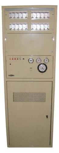
In common with all of the current Drallim pressurisation units. the 12255 will dry the output air to а minimum dewpoint of -40°C. The standard humidity detection equipment within the unit ensures that. problem should а occur, any moist air will be exhausted to atmosphere rather than being allowed to enter your cables. Sound-proofing is а standard feature of the
