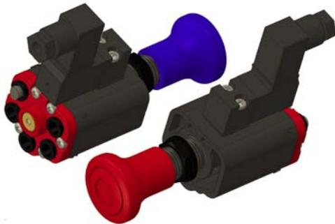
**The Electrical Release (SP):** The SP valves require an electrical signal to the integral solenoid valve before the valve may be operated. In the absence of the electrical signal the valve remains closed and the control knob locked, making it ideal for interlocking with hand-brake electrical control circuits for additional safety.
