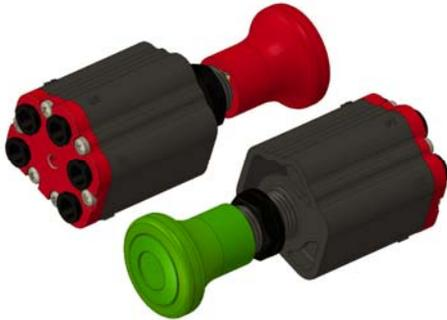
**The Manual Air Release (AR):** The AR valves require the air signal to be removed/disengaged from the reset port before the valve may be operated. When the reset signal is restored the valve is returned to the closed position and the control knob locked, making it ideal for interlocking with hand-brake air systems for additional safety. The valve may also be used as a 4/2 valve when no reset signal is required.
