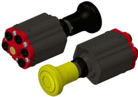
**The Manual Air Applied (AP):** The AP valves require an equalising pressure signal to be applied to the reset port before the valve may be operated. In the absence of this signal the valve remains closed and the knob locked. These valves are particularly suited for use in Fuel-tanker discharge systems as Master or Foot-valve controls.
