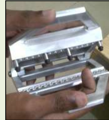
SIMPLE FIXTURE FOR STEEL PLUNGER AND RUBBER CAP ASSEMBLY
