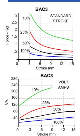
**AC Closed VA** 100% Rtg = 9VA 50% Rtg = 20VA 25% Rtg = 40VA
