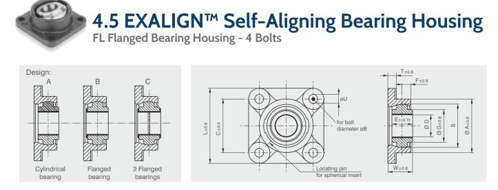
Housing material: GG 20 Spherical insert material: GG 20
