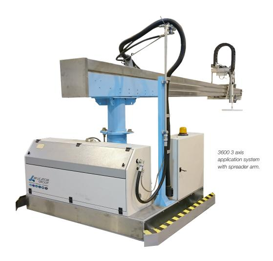
System 3600 mixes and dispenses adhesives and resins such as polyur ethane, epoxy and ms-polymers. The automatic system is the perfect choice for sandwich panel manufacturing, when there is a
