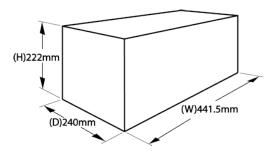
Whether you choose the 230vAC or the 48vDC variant, the 12446 boasts an impressive output of over 220 litres per hour at an excellent dewpoint of -40°C. The unit comes with 2 fixed output pressure options of either 15 or 40 mbar, and 6 off ½" pneumatic outlets as standard.
