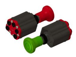
The Manual Air Release (AR): The AR valves require the air signal to be removed/disengaged from the reset port before the valve may be operated. When the reset signal is restored the valve is returned to the closed position and the control knob locked, making it ideal for interlocking with hand-brake air systems for additional safety. The valve may also be used as a 4/2 valve when no reset signal is required.
