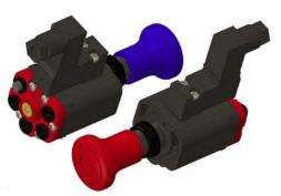
The Electrical Release (SP): The SP valves require an electrical signal to the integral solenoid valve before the valve may be operated. In the absence of the electrical signal the valve remains closed and the control knob locked, making it ideal for interlocking with hand-brake electrical control circuits for additional safety.
