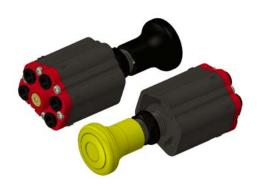
**The Manual Air Applied (AP)**: The AP valves require an equalisng pressure signal to be applied to the reset port before the valve may be operated. In the absence of this signal the valve remains closed and the knob locked. These valves are particularly suited for use in Fuel-tanker discharge systems as Master or Foot-valve controls.
