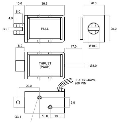
2 X M3X0.5 FIXING HOLES BOTH SIDES OF FRAME
